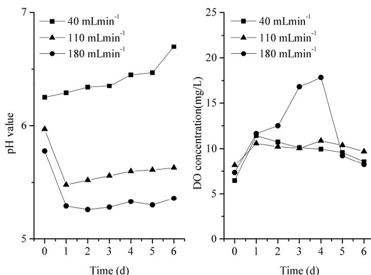
Fig.4. pH value and DO concentration curves in CRWP aerated with different gas flow rate
