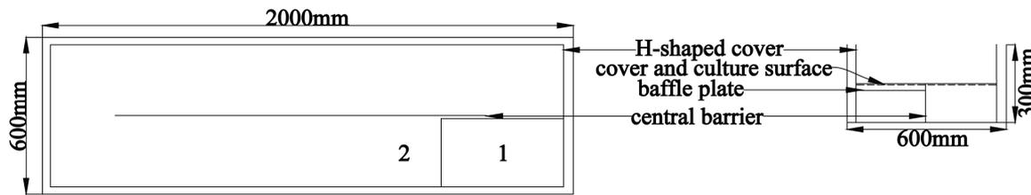
Fig.1. The schematic of closed raceway pond
